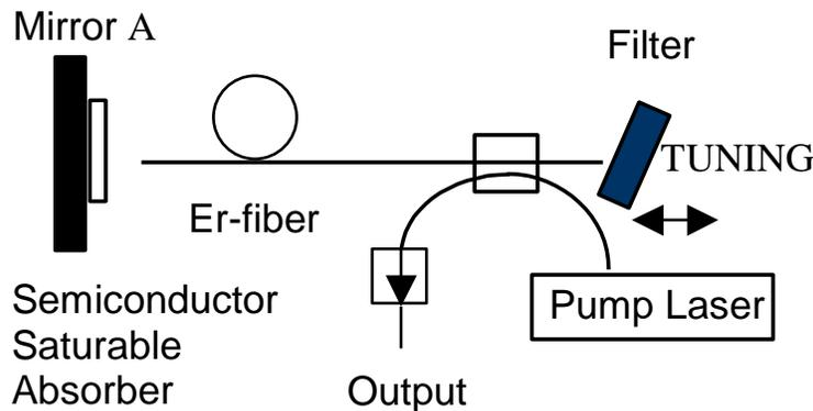
**Figure 1 – Schematic of Passive Mode-locked Fiber Laser**
