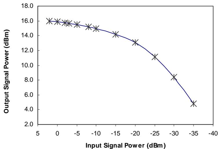
**Figure 3 – Output Power vs. Input Power (AMP-LD-15)**
