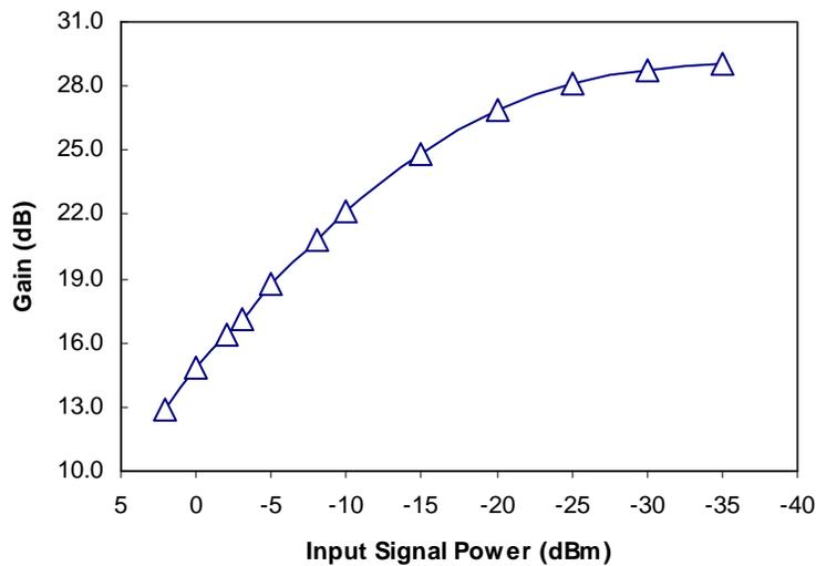
**Figure 2 – Gain vs. Input Power (AMP-LD-15)**
