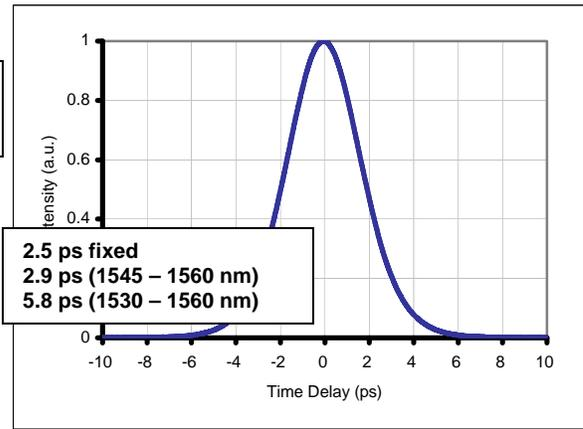
**Figure 3 - Pulse Width FWHM of 2.5 ps (Calmar PSL-10-2)**
