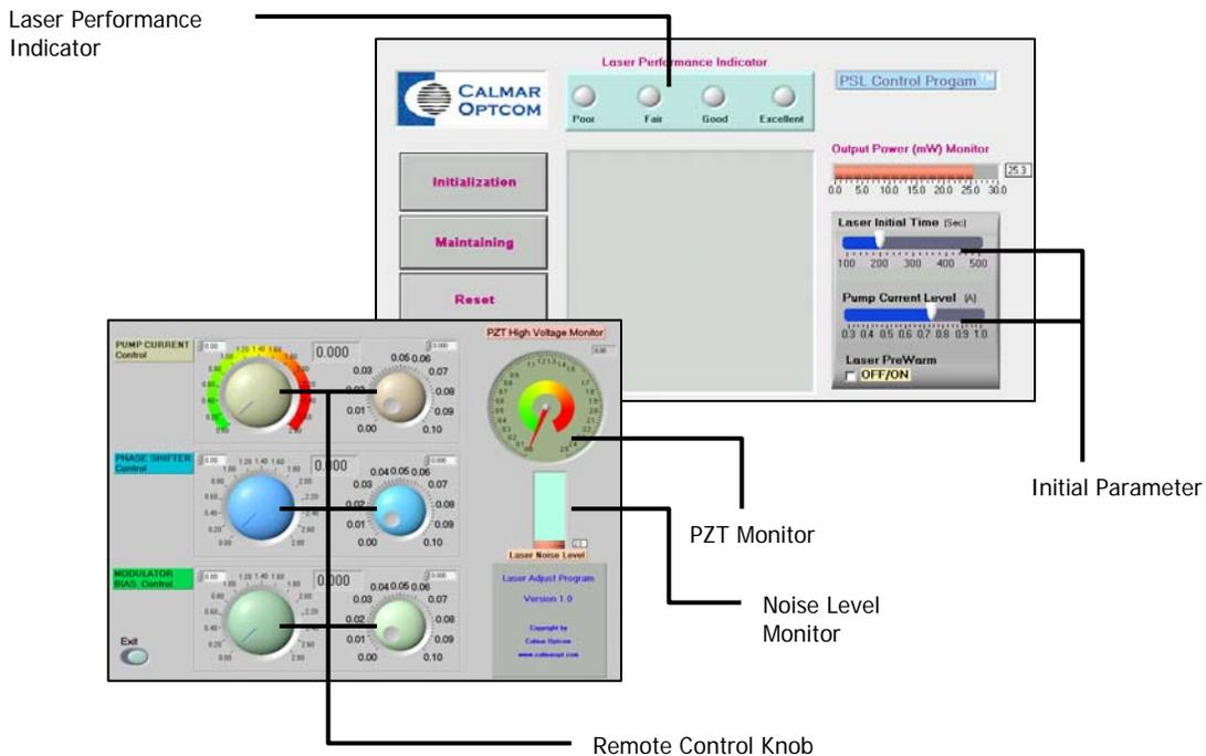
**Figure 13 - Remote Control Interface**
