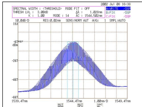
**Figure 5 – Spectral Width of 1.0 nm (Calmar PSL-10-2)**
