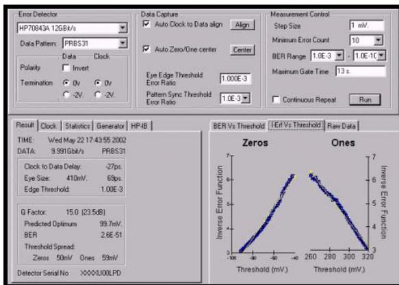
Figure 11 – Q and Eye Analyzer Results
