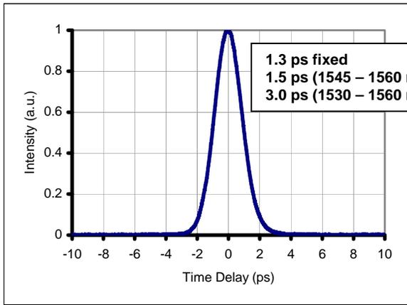
**Figure 2 - Pulse Width FWHM of 1.3 ps (Calmar PSL-10-1)**
