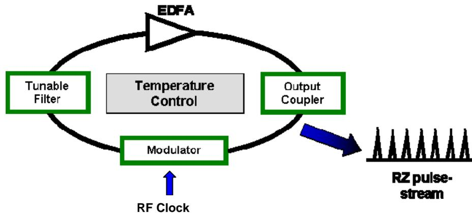
**Figure 1 - Simplified Schematic for a Fiber Laser**
