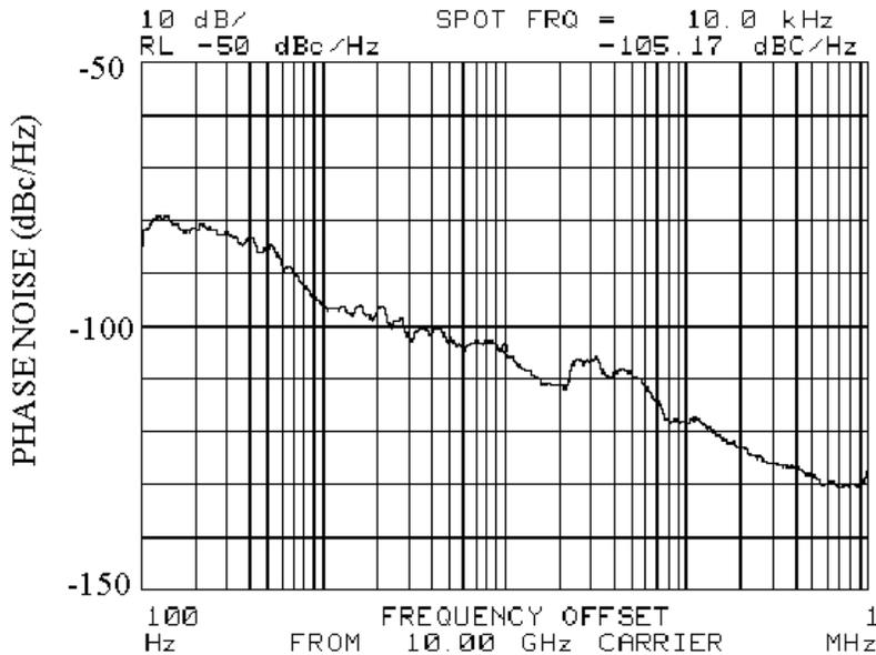
**Figure 8 - Timing jitter of 45 fs**
